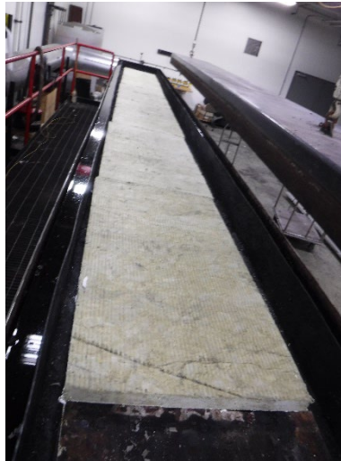
Photo No. 3 Unexposed Surface of the Test Specimen (Pre-test)
